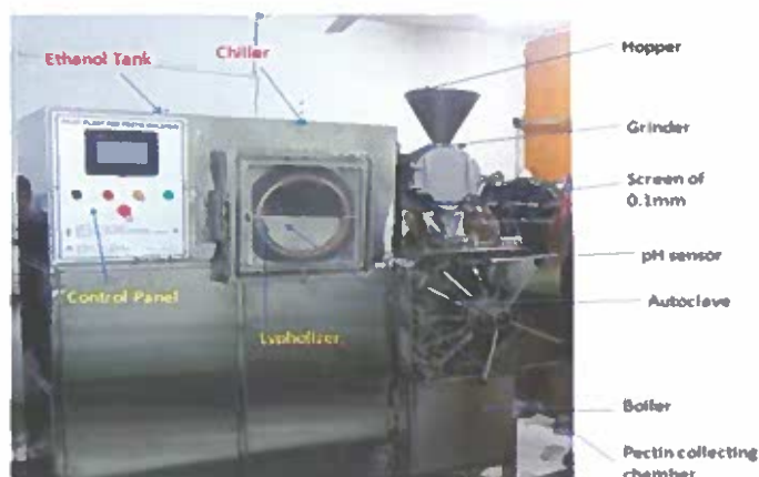
Pilot plant for pectin extraction
